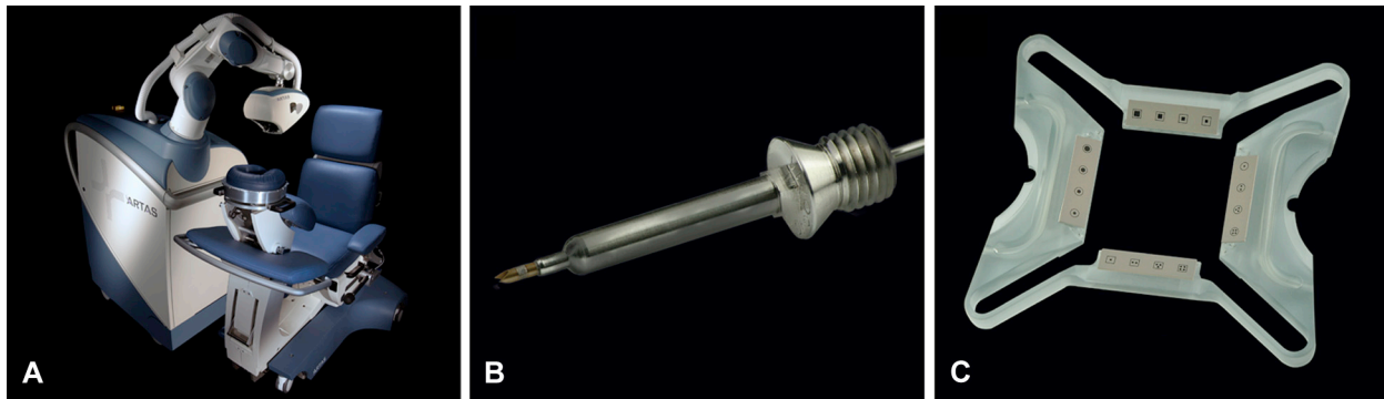
Fig 1. ARTAS robotic system (Restoration Robotics Inc, San Jose, CA). A , The system is composed of a cart with an articulated robotic arm and a specialized chair. B , Dissection system with a needle-in-needle configuration in which a sharp bi-beveled needle (inner needle) is concentrically arranged within a blunt outer punch. C , A classic tensioner. (Printed with permission from Restoration Robotics Inc.)
